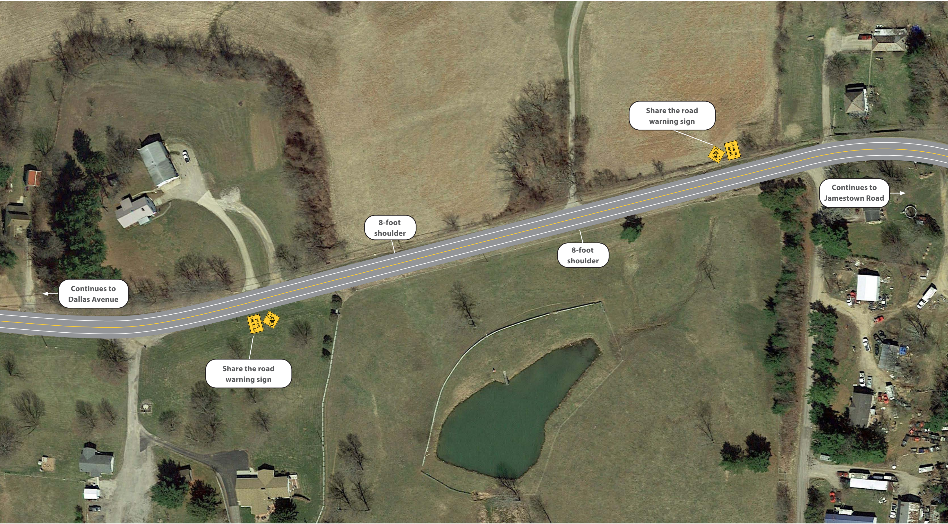
Figure 8. State Route 13/37/93 Paved Shoulders Conceptual Design (RR4C)
