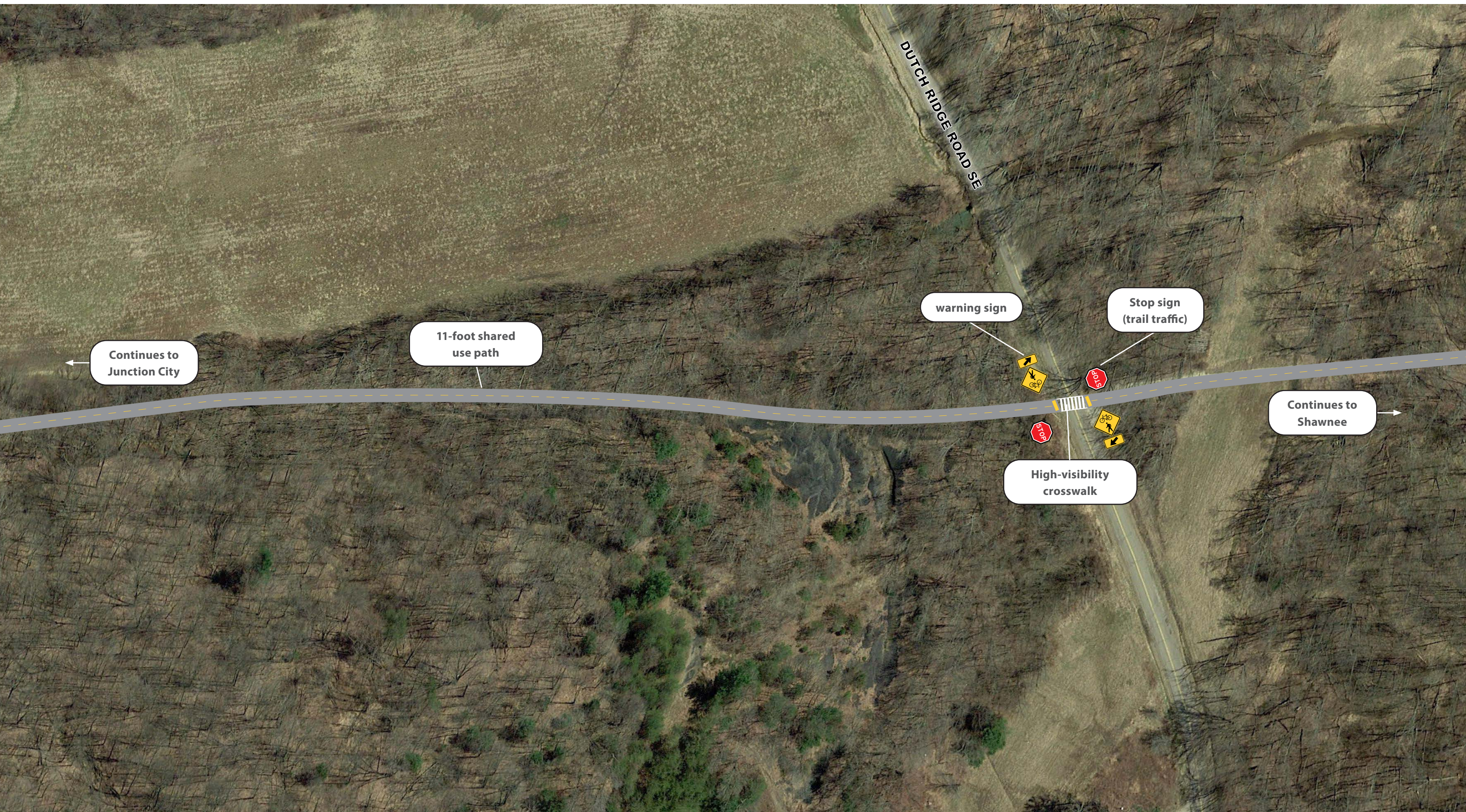
Figure 9. Shared Use Path from Shawnee to Junction City Conceptual Design (RR2C)
